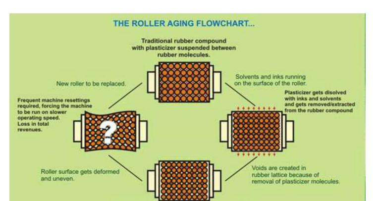
Leads to shrinkage in diameter and increase in hardness.
